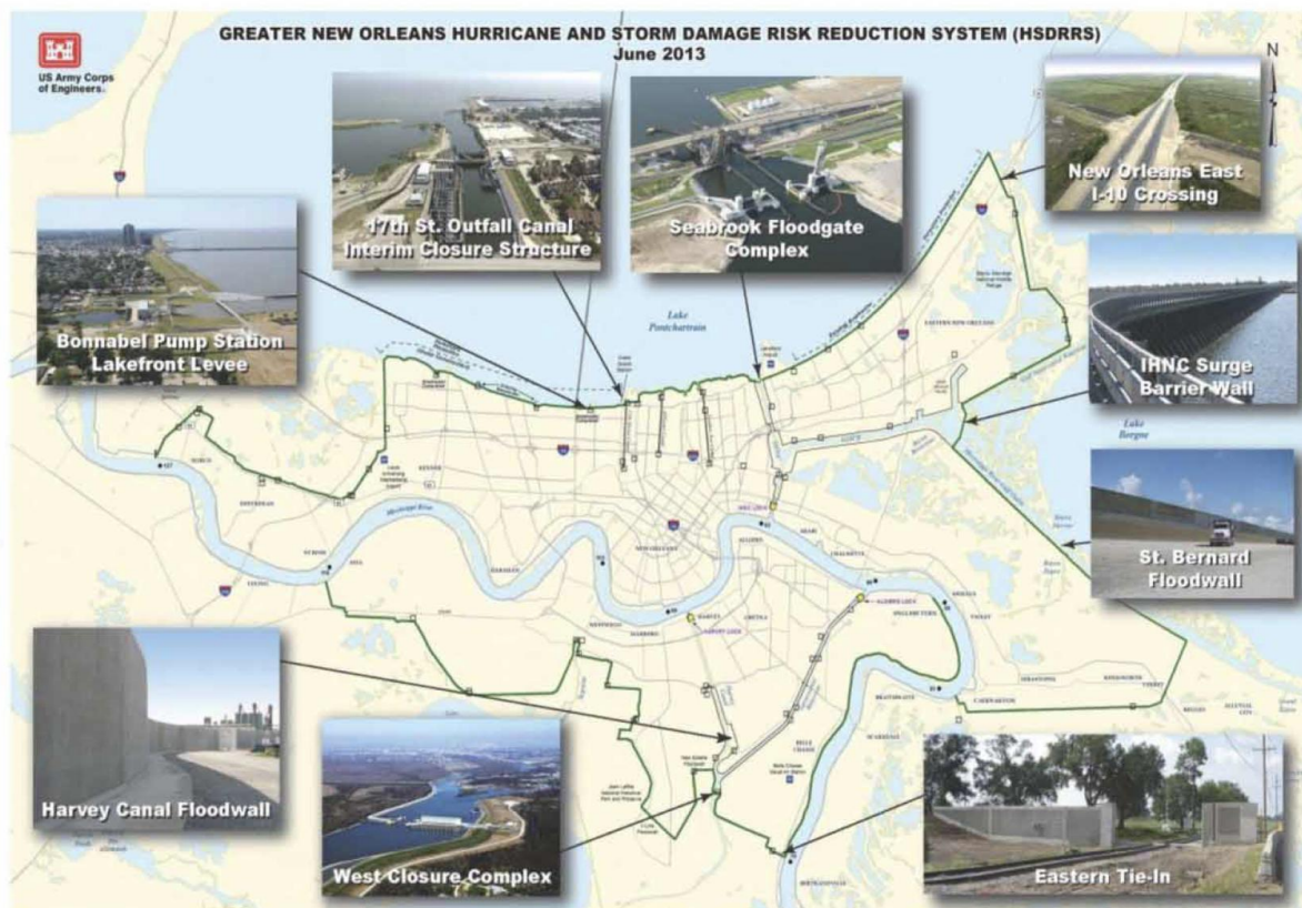
Figure 4. Map showing the major components for the Hurricane Storm Damage Risk Reduction System. This included considerable improvements and elevation of existing levee and floodwall sections that did not fail during Katrina. (Source: U S Army Corps of Engineers)
