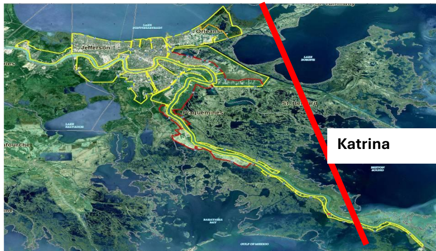
Figure 1. Graphical depiction of the hurricane protection system in New Orleans prior to Katrina and showing Katrina's path. The yellow lines show federal levees and structures and the red show non-federal levees. A good portion of the structures in the upper left portion of the graph were incomplete when Katrina struck. (Source: IPET)
