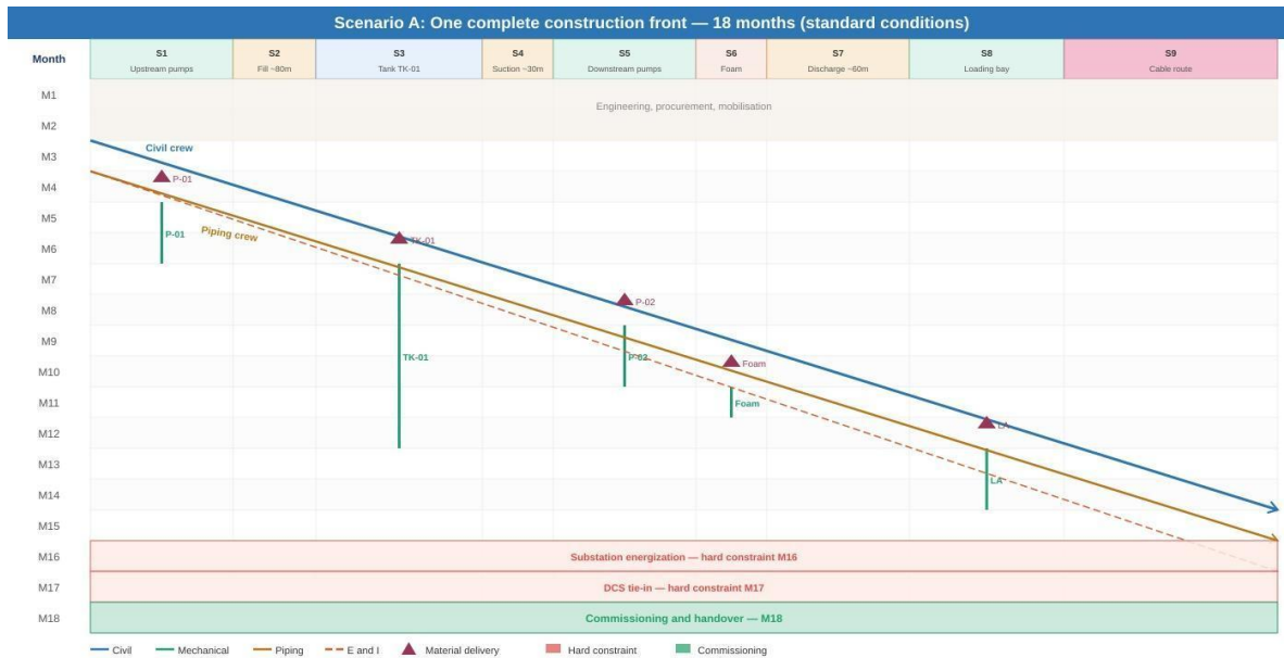
Figure 3a: Scenario A, product loading facility. One complete construction front, 18 months. Sequential material delivery, single crew movement left to right across all sections.
