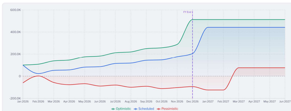
Figure 1: A project with an initial payment, then regular payments, and a final payment for success is in two scenarios consistently profitable for the contractor. 4
