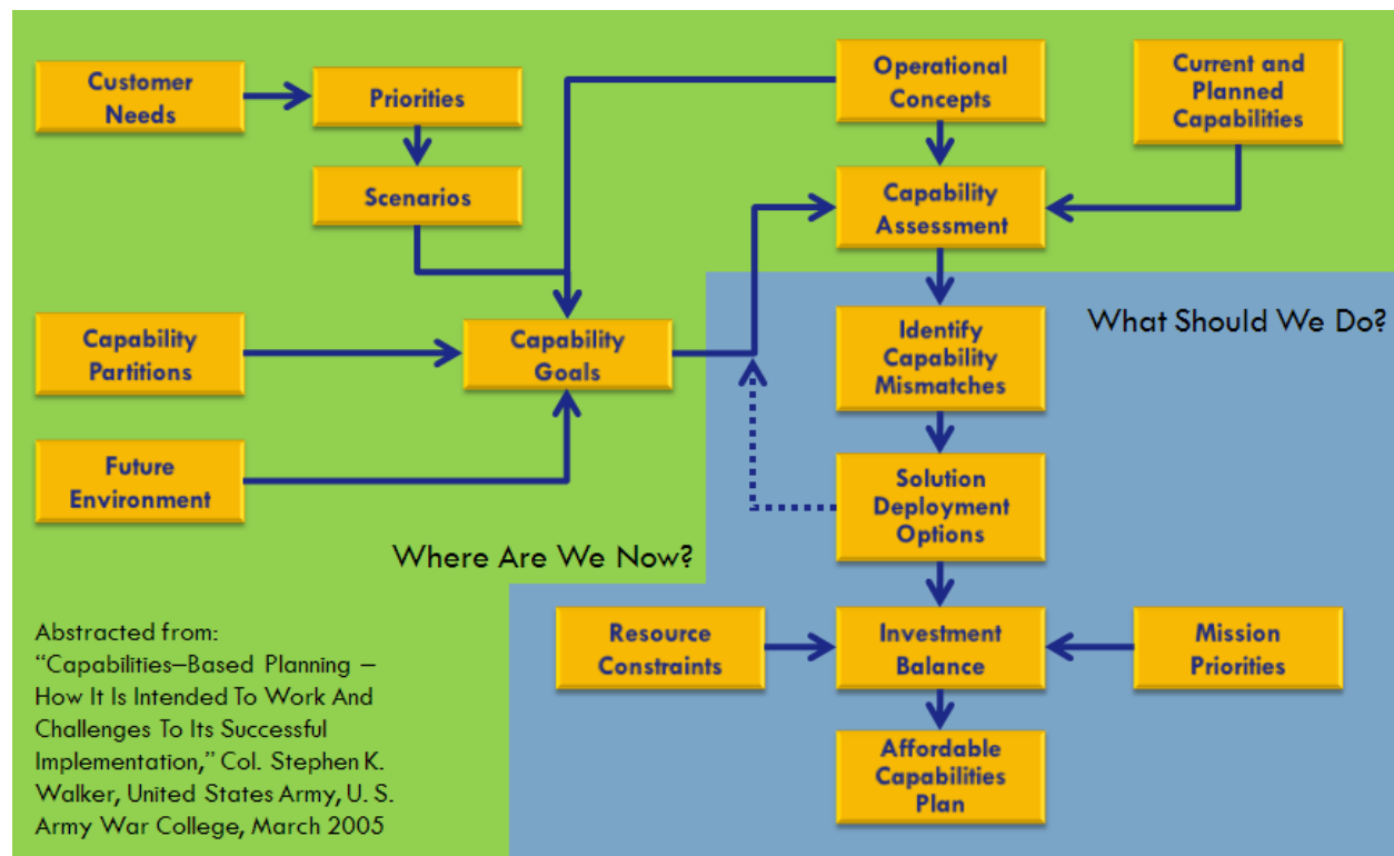
Figure 2 – Capabilities Based Planning starts with identifying customer needs through scenarios rather than technical requirements. This approach answers why I want this and what I will do with it when I get it . The Concept of Operations (ConOps) contains scenarios implementing the needed capabilities. With the ConOps, the requirements are derived that fulfill each Capability. Then can each requirement have a reason for being present?
